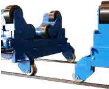
Welding rotator on rails
