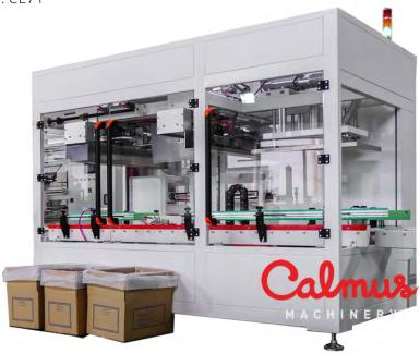
This is a fully-automatic poly bag inserter | carton liner placer, made in China. It is designed for lining cartons with polybags by one each. This **poly bag inserter** cuts and seals film as a bag from a roll stock, inserts it in a formed box, opens and cuffs the bag over the carton top flaps, blows air to extend the bag to fit the internal wall of box better.
